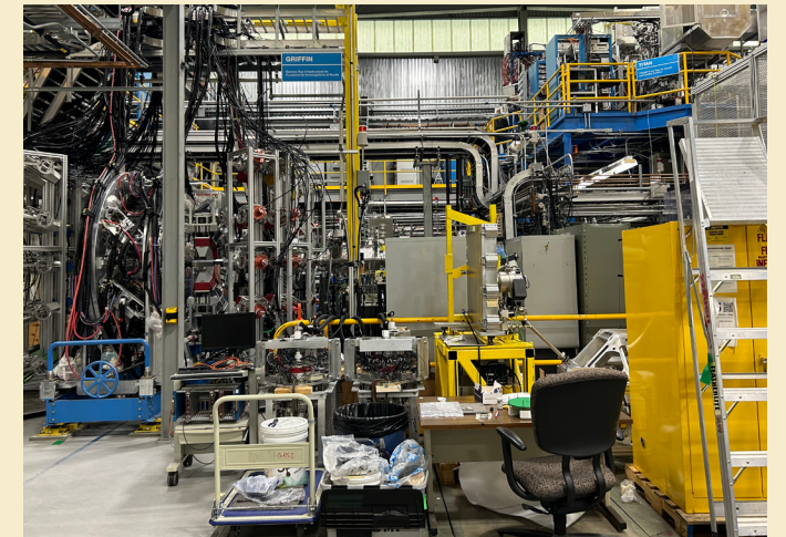
The floor of the ISAC 1 building at TRIUMF. Here, we can see the GRIFFIN experiment, which investigates nuclei with gamma rays, the TITAN experiment, which measures the mass of short-lived isotopes, and off to the right is the \beta -NMR facility, which detects an NMR spin precession signal through beta decay of a radioactive isotope.
