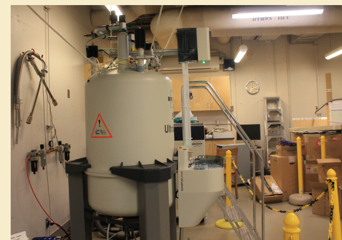
The chemistry department's 500 MHz NMR spectrometer, surrounded by a barrier indicating the safe distance from the spectrometer's magnetic field.
