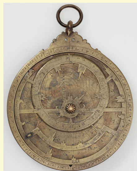
Ninth century astrolabe, which uses the law of sines to make astronomical predictions.
